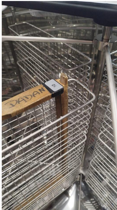
Fig. 7.1. Correct positioning of frames in a cassette honey extractor (WL, OS, D, LN. AP) Designations: WL-Wielkopolska, OS-Ostrowska, D-Dadant, LN - Langstroth, AP - Apipol
